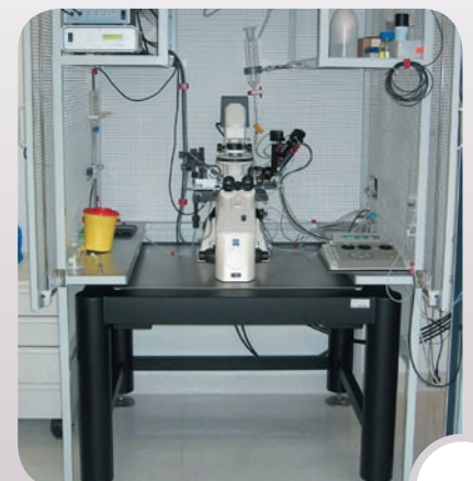
▶ Active Workstation 900 with patch-clamp setup inside a Faraday cage.
